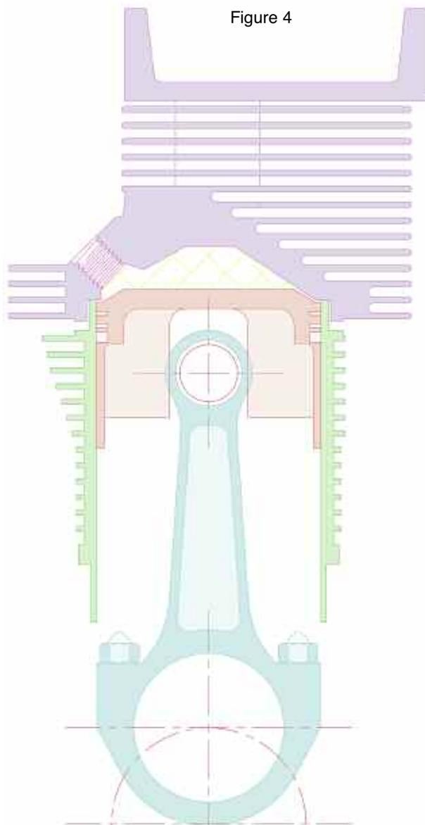
height volume. It is the volume represented by the deck height (the distance from the deck of the piston to the top of the cylinder) times the piston area. Since this example is based on 'big bore' pistons with a radius of 43mm, good, old Pi R squared times the 1mm deck height means a net chamber volume of 5.8cc.
